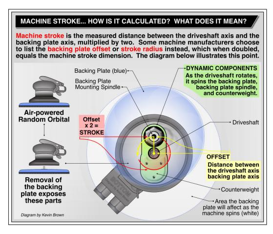
Machine manufacturers also refer to machine offset using terms such as backing plate offset, stroke radius, and stroke diameter. Regardless the terminology, these terms are all identifiers of the machine's movement.
