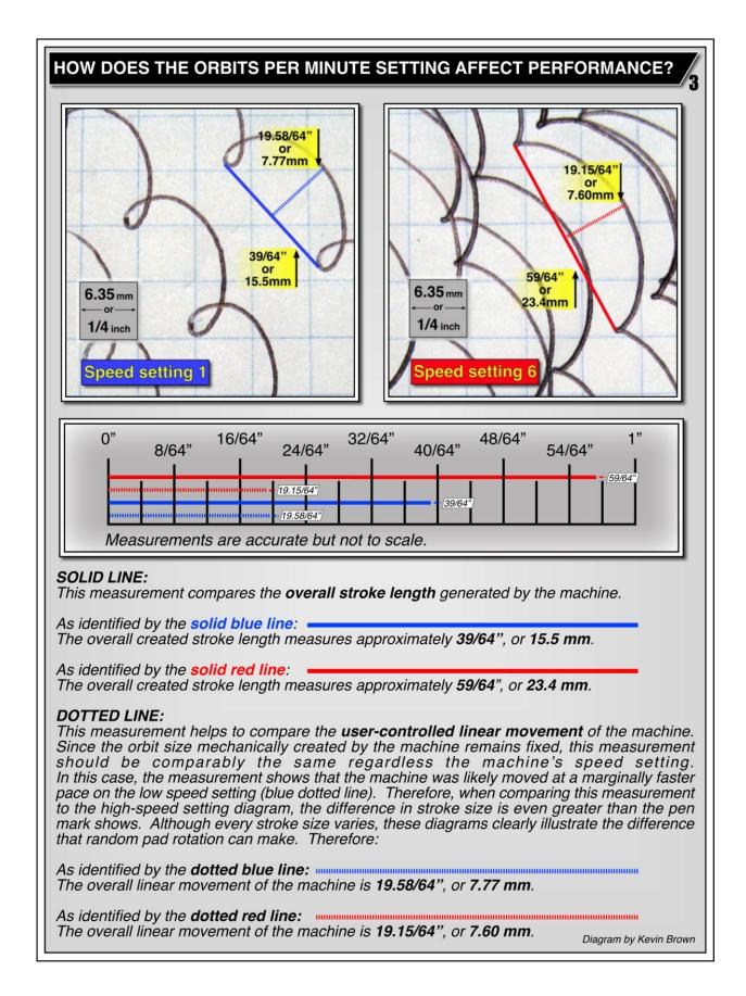
Keep in mind that in terms of **leveling** a large surface (one that is larger than the diameter of the pad), there is no denying that a *large diameter disc* will level that surface *more consistently* than a *small diameter disc*. Since this article pertains to machine stroke, how best to illustrate the performance differences between small and large stroke machines? A comparison of *machine stroke* to a typical *handheld sanding block* helps to illustrate the point:
